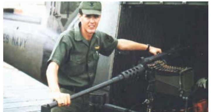
A .50-caliber machine gun is mounted on the right side, paired with twin M60s on the left side to give the Huey lethal firepower.
