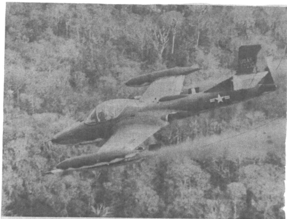
A-37 aircraft of the 8th Special Operations Squadron, under the 315th Tactical Airlift Wing, are designed to meet specific requirements of the Air Force for counterinsurgency operations and close air support for ground forces in Southeast Asia. The maneuverability of the aircraft at a relatively low rocket-firing and strafing speed allows it to "press in" to a target for greater delivery accuracy. (USAF Photo)
