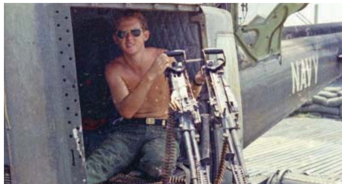
A .50-caliber machine gun is mounted on the right side, paired with twin M60s on the left side to give the Huey lethal firepower.
