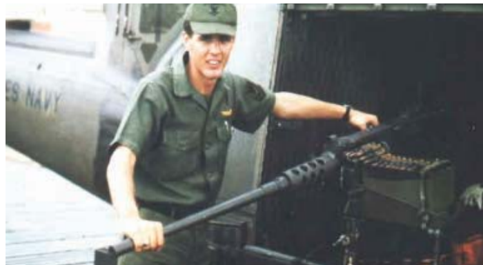
A .50-caliber machine gun is mounted on the right side, paired with twin M60s on the left side to give the Huey lethal firepower.
